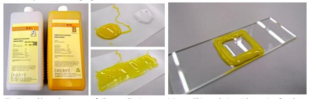
Tip: Try and keep the amount of silicone adhesive to a minimum. This results in quicker setting & reduces the chances of the objective lens pushing against the silicone when imaging.
