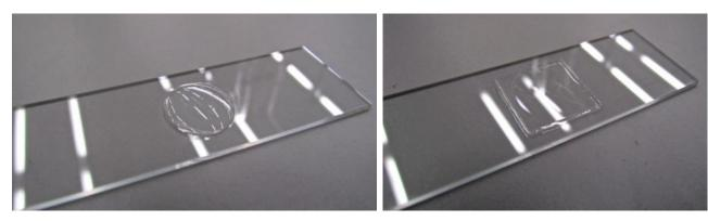
2. Mix silicone adhesive components A and B together in a 1:1 ratio and then carefully apply with a cocktail stick around the edges of the coverslip. Wait 15-30 minutes for it to set firmly before imaging.
